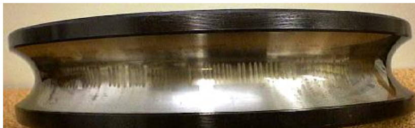
Figure 18 – ‘Characteristic ‘fluting’ wear of inner race
